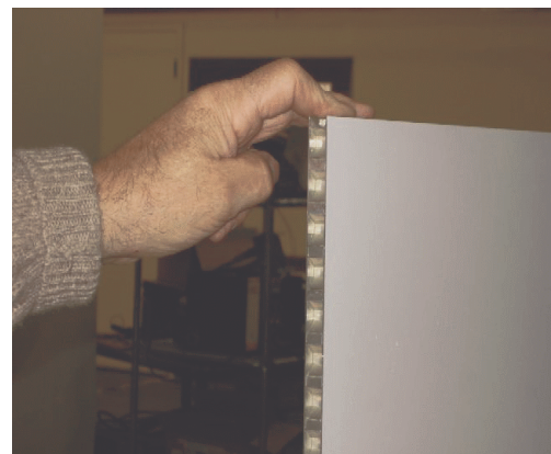
Honeycomb structural panel.
